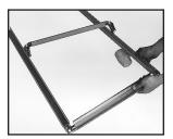
Slide two longer angle pieces onto corner pieces already inserted into shorter pieces, then add the second short piece to complete the frame.
